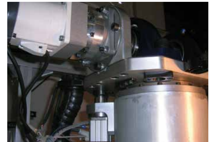
The iglidur® PRT-01-100 slewing ring is used in an automatic welding plant in this application. It enables pivoting in the horizontal plane of the clamping device.
