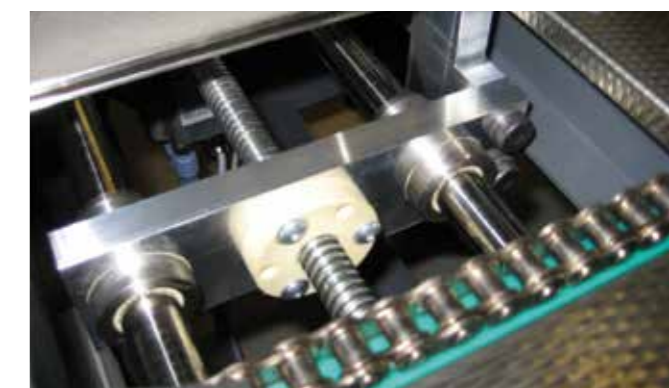
Format adjustment in the paper industry with anti-backlash lead screw nut
