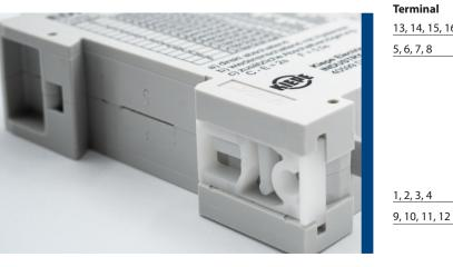
The top hat rail enables quick and easy mounting of the switch in the existing control cabinet. The speed monitor is first placed on the top hat rail with the mounting edge and then pressed onto the top hat rail until the catch engages.
